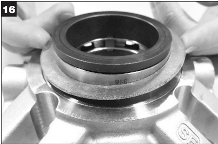
Remove the gasket from the adapter and discard.
