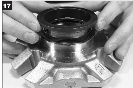
Remove the inboard stationary seal ring from gland and discard.
